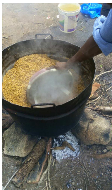
Figure 13. Steam parboiler; Traditional parboiling pot.
