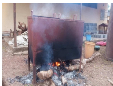
Figure 12. Steam parboiler; Improved parboiling pot.
